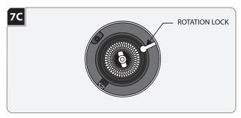
**NOTE:** Lamp housing can rotate 361° horizontally.
